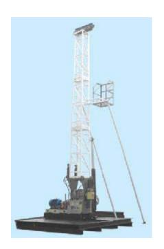
drilling vertical as well as inclined holes. The range of adjusting angels (in clock-wise direction) for drilling inclined holes is  $0^{\circ}$ - $90^{\circ}$ .
